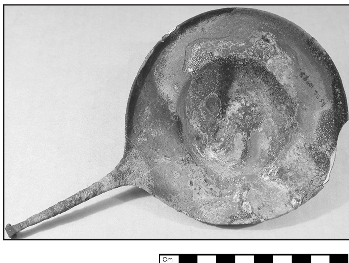
Figure 4. Copper alloy sieve OIM A11273 from Tell Asmar, Iraq, with most abundant occurrence of unusual corrosion, covering 25% of mineralized surface
