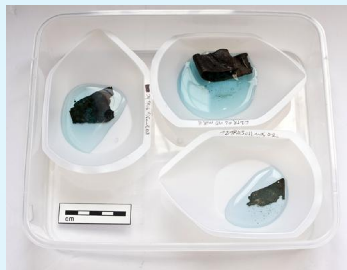
Figure 4. Though no surface changes were observed, the EDTA solution did change color (from clear to blue or green) during immersion of some of the bronze objects, such as with these metals from Kerkenes Dağ. This indicates that other components, in addition to lead, have been extracted and gone into solution.
