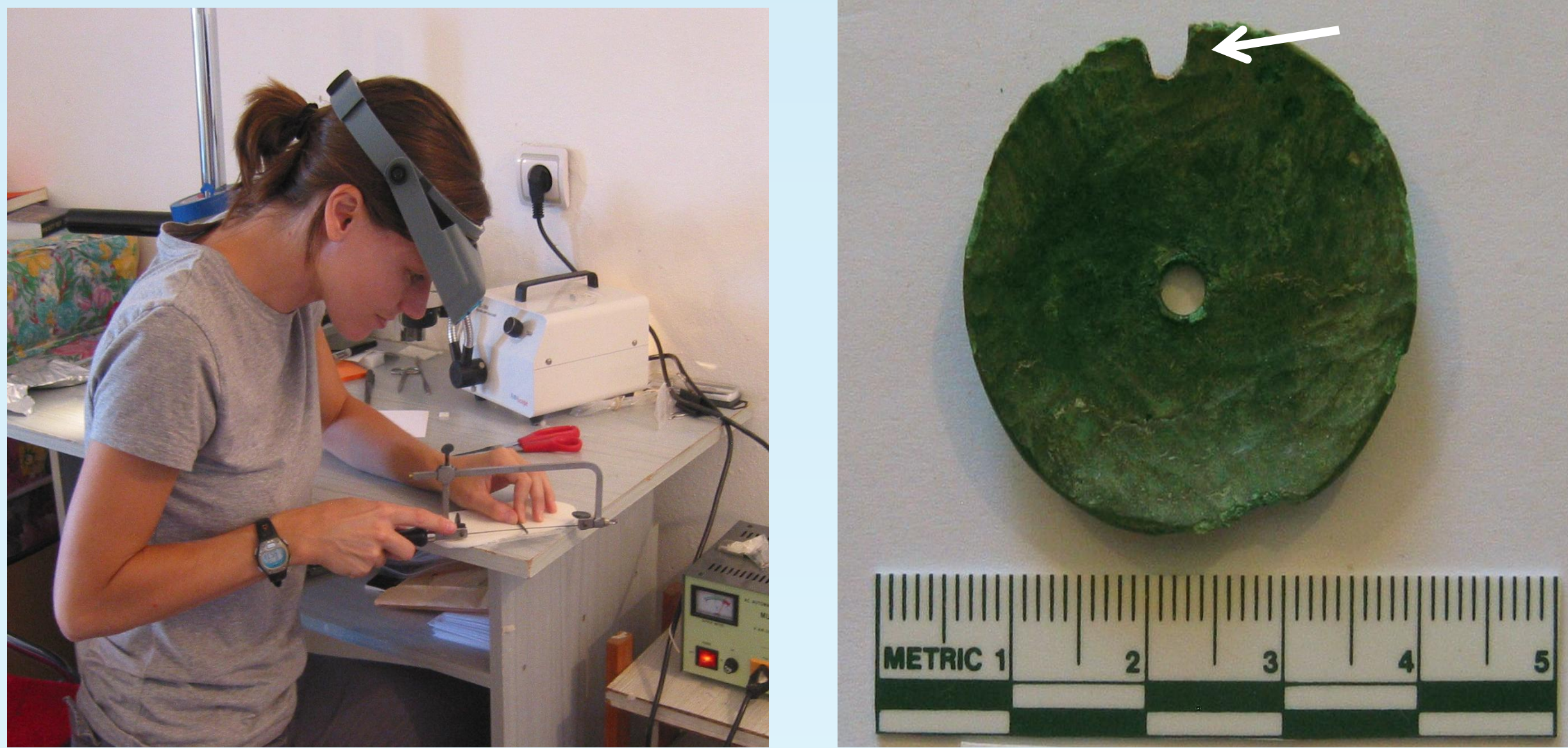
Figure 1. Sampling a bronze disc from the site of Lofkënd using a jeweler's saw (left). Sampling required a small piece from the edge of the disc to be taken (right).
